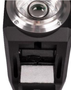
Figure 65: Inlet filter replacement
